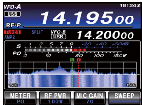
Spectrum Scope Display (Waterfall Mode)
